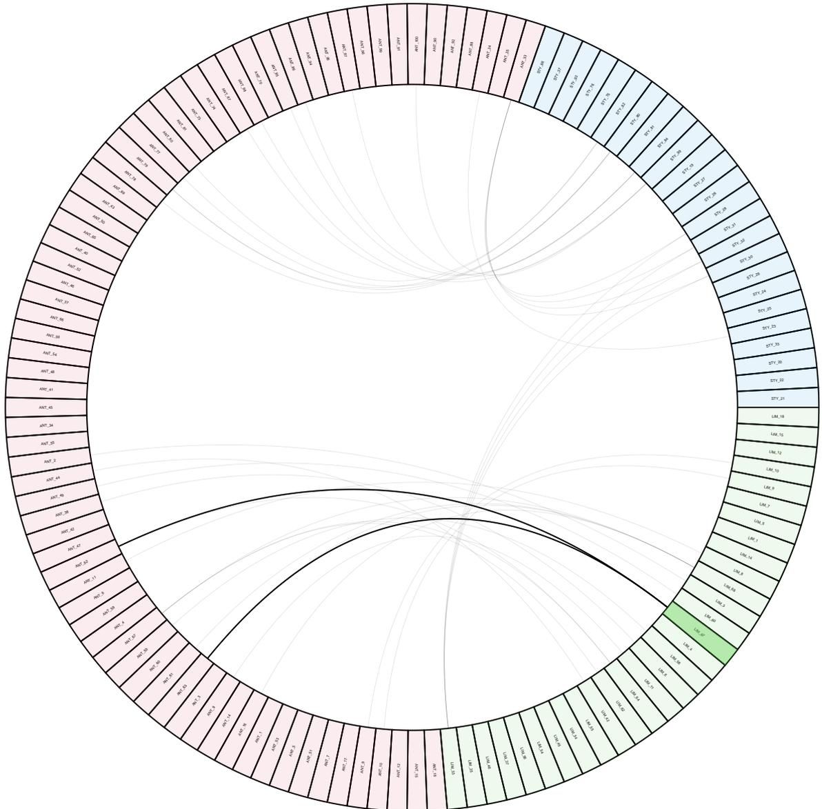
Figure 2: Exemplary circos plot highlighting an arbitrary feature. Upon highlighting, all links will be plotted in grey (expect links to and from highlighted features). The intensity of the background colour of features will be reduced as well. Features belonging to a group (species, individual, organ, different time) will be indicated by the same background colour.
