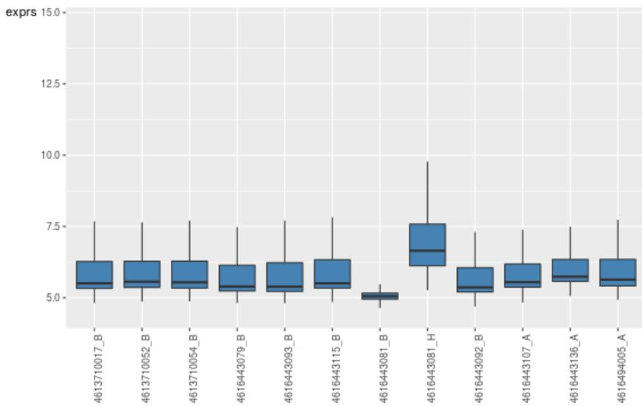
In a similar manner, we may wish to visualize the differences between sample groups for particular probe groups. As a simple example, we look at the difference between negative controls and regular probes for each array. You should notice that the negative controls as consistently lower (as expected) with the exception of array 4616443081\_B.
