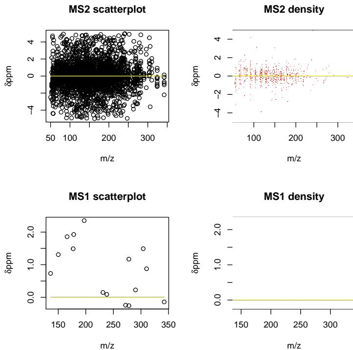
The recalibration graph shows that the recalibration "curve" will do no recalibration. To verify, we can show the same peaks as before:
