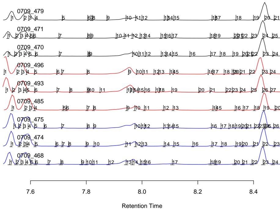
Note here the little *hashes* represent the detected peaks and are labeled with an integer index. One of the main challenges is to match these peak detections across several samples, given that they appear at slightly different times in different runs.
