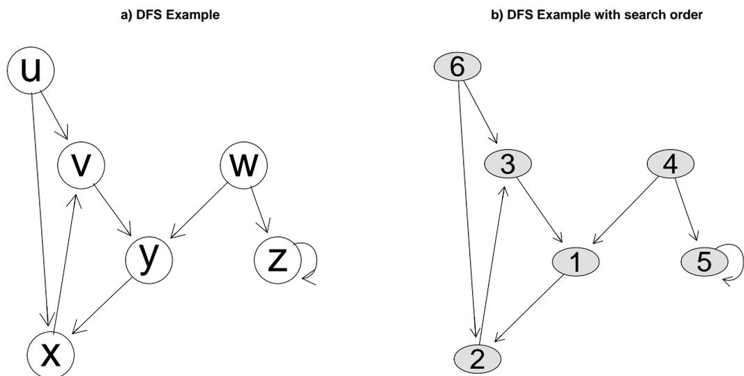
Figure 5: a) The graph for depth-first-search example. b) The graph for depth-first-search example, showing search orders.
